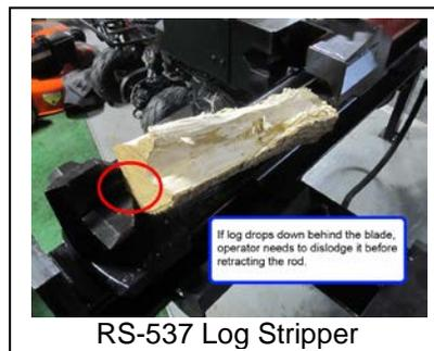
Your log splitter is very powerful. Do not allow pieces of wood to become lodged behind the horizontal blades of the RS-537. Retracting the rod when a log is jammed behind the blade may damage the log stripper and the valve. The heavy duty log stripper will strip normal sized pieces of split wood off of the blade, but it is not designed to
